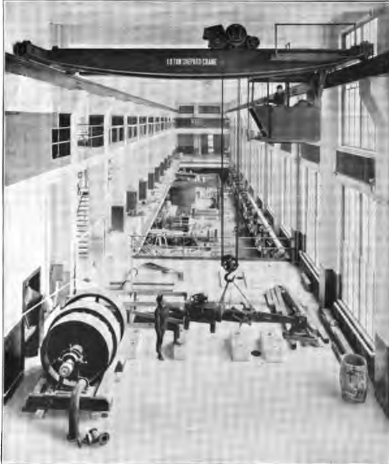
Fig. 162. Electric Traveling Crane in the Hydraulic and Steam Laboratory of the Massachusetts Institute of Technology, 1916.
